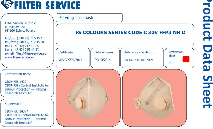
Protection of human airways against harmful airborne solid particulates and/or liquids in aerosols (dust, smoke and mist) at a maximum exposure level of 30 times PEL (Permissible Exposure Limit).
