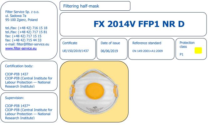
Protection of human airways against harmful airborne solid particulates and/or liquids in aerosols (dust, smoke and mist) at a maximum exposure level of 4 times PEL (Permissible Exposure Limit).
